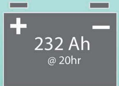
Amp hour ratings are often used to compare batteries, but not all Ah ratings are taken at the same discharge rate (10-hr, 20-hr, etc.). Batteries that show the same ratings may be completely different, as the advertised discharge rates may be higher for one rating and lower for another.
